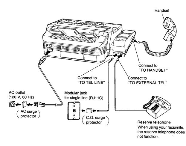
The unit including the telephone handset will not function during a power failure or power off. However, if you have a reserve telephone connected to the port of the "TO EXTERNAL TEL", you will still be able to make calls during a power failure or power off.
