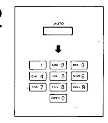
Press the AUTO button, then press the desired speed dial station number (00 through 99) by using the dial keypad.
