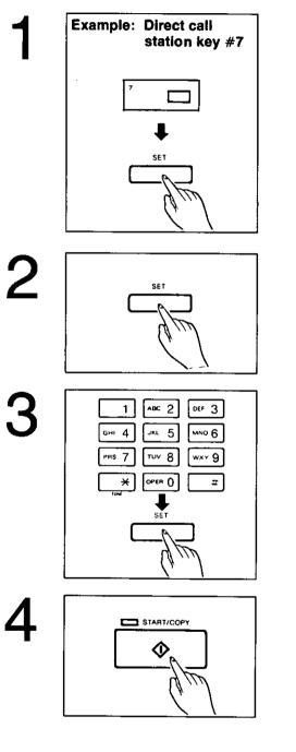
Enter the desired phone number using the direct call station key or the speed dial station, then press the SET button. (Example: Direct call station 7 is dialed.)
