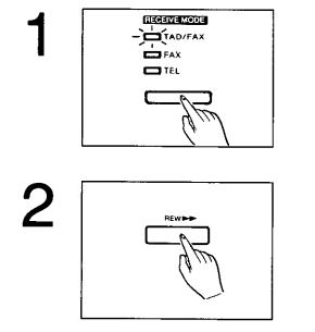
Press the RECEIVE MODE button until the TAD/FAX indicator lights.
