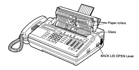
If you cannot get a clear copy after performing the above steps 1 and 2, clean the thermal head with a cloth moistened with denatured alcohol (alcohol without water), then dry thoroughly. To prevent malfunction due to static electricity, do not use a dry cloth and do not touch the thermal head with your finger directly.
