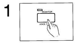
Press the MONITOR button or lift the handset.
