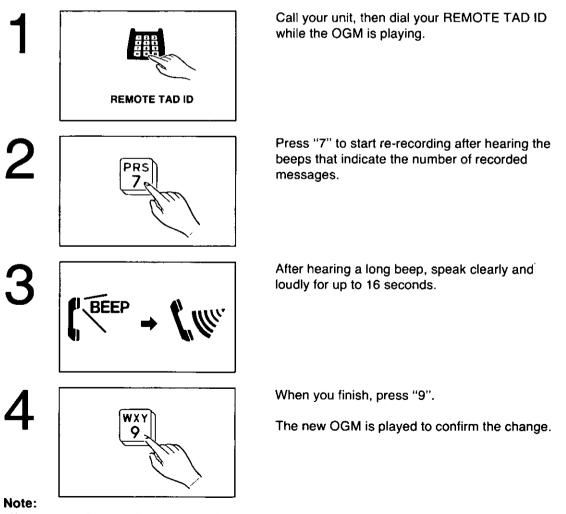
•If you pause for over 2 seconds while recording, the unit beeps and stops the OGM recording. In this case, repeat from step 2 within 10 seconds.
