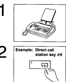
Press the desired direct call station key. (Example: Direct call station 6 is dialed and its name is Panasonic.)
